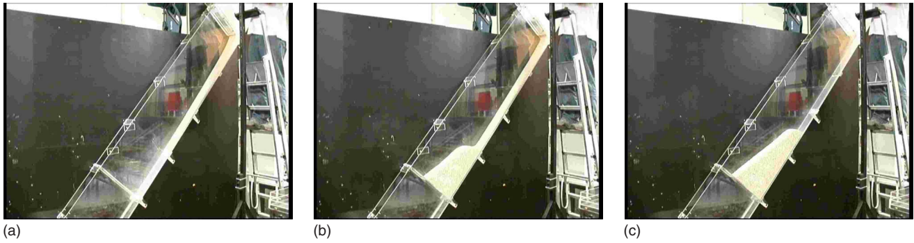
FIG. 2. (Color online) Laboratory experiments of dry granular chute flows impinging an obstructing wall. Granular material is continuously released by opening the shutter of the silo (a). The material then moves rapidly down the chute and impinges on the obstructing wall forming shock (b). This leads to a sudden change in the flow regime from a fast moving supercritical thin layer to a stagnant thick heap with variable thickness and a surface dictated by the angle of repose typical for the material. Final deposition is shown in the (c).
